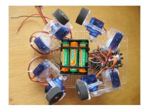
This robot works best with a small LiPo battery (7.4V, 2300mAH) but rechargeable AA NiMh batteries are more common and easier to recharge so we will use 6x AA NiMh batteries for these instructions. Do not use alkaline batteries, the voltage is too high and they cannot put out enough current to drive the servos. This will cause your processor to continually reset. Use good quality batteries with at least 2000mAH capacity.
