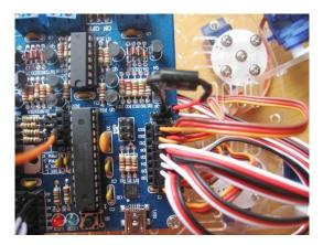
Start by fitting the servo extension cables to the front leg servos. Now plug in your leg servos.
