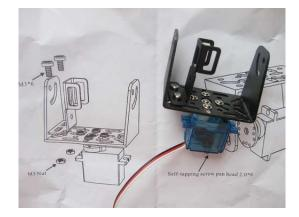
The tilt servo locating bracket doesn't actually hold the tilt servo in place. It's main purpose is to prevent the tilt servo from twisting while allowing some play so the servo can self center.
