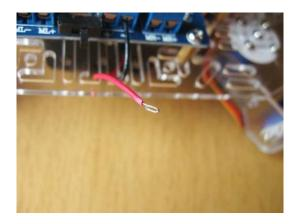
Make sure the power switch is in the off position and then remove the tape from your black (- negative) wire. strip the wire back, twist the strands together and then bend it over before inserting into the screw terminal as shown in the photo. This will help to ensure a good connection. Now remove the tape on the red wire (+ positive) and do the same.
