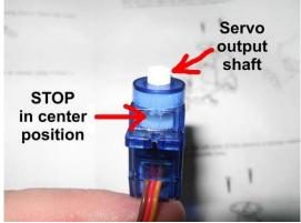
The QuadBot chassis kit includes 8x miniature servos and the Pan/Tilt kit includes 2 miniature servos. These servos have clear cases so you should be able to see through them well enough to check that they are centered.
