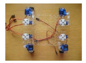
The mounting plate of the QuadBot chassis is the laser cut acrylic panel that you mount all your parts on. Mount your left and right legs as shown in the photo.
