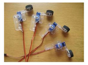
Once you have mounted the servo horns on the thigh segments they can be attached to your knee servos using 4 of the 8 supplied 2 x 8mm pan head screws. With your knee servo centered the thighs should be at 90 degrees to the leg segment with the foam rubber foot.
