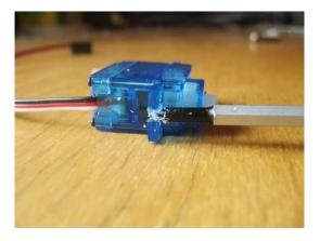
The brass hex spacers used to mount the pan / tilt kit require a 3mm screw but the miniature servo housing has a hole designed for a 2mm screw. Previously I have tried using a 3mm drill bit but it bites into the plastic which can break the servo mounts and it can accidently dig into the servo cable.
