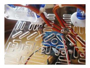
Use two 3 x 10mm pan head machine screws to mount the head. Notice the holes used in the first photo. The servo is mounted slightly toone side so that the pan servo's output shaft is centered rather than the servo body. The pan servo is mounted a reasonable distance back to improve the ballance of the robot and to help protect the pan servo if the robot runs into a wall.
