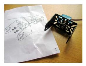
The pan / tilt kit comes with two large brackets. Each bracket has a different hole pattern on it to suit many different sensors. Look at the photo below and make sure you attach the correct bracket to the pan servo as the compound eye cannot be mounted if you use the wrong bracket.
