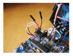
Connect your pan servo to A4 and your tilt servo to A5 with the white signal wire towards the female header. The software reconfigures these pins as servo outputs.
