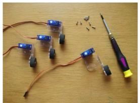
Mount 4 of your servos on the leg segments with the foam rubber feet. Use 2.3 x 8mm self tapping screws.
