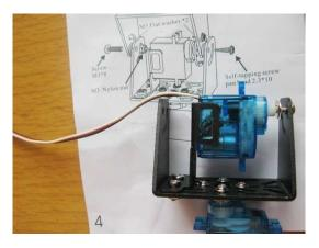
Use a 2.3 x 12mm screw to align your tilt servo. The servo will be a firm fit in the tilt servo locating bracket. Adjust the position so that the servo alignes with the pan bracket and allow room for spacer washers and a servo horn. Once everything is aligned you can tighten the 3mm screws holding the tilt servo locating bracket so that it wont move.
