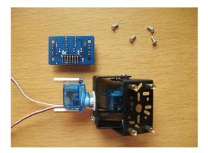
The IR compound eye is a simple sensor that measures ambient light and reflected IR light from an object. The eye has seven connectors. Vcc (+5V) and Ground for power. The ENable pin turns the IR LEDs on or off and then there are 4 analog outputs for up, down, left and right.
