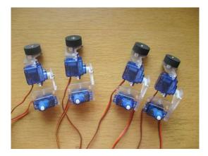
So far all of your legs should look identical. Now we will seperate them into left and right legs. The only difference between a left leg and a right leg is the way in which the thigh servo is mounted.
