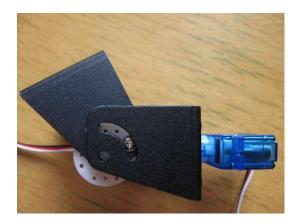
There are some spacer washers that must be inserted so that the tilt assembly can rotate smoothly. The easiest way I know to insert these spacer washers is to lie the pan / tilt assembly on it's side with the tilt bracket at about 40 degrees when the tilt servo is centered as shown in the first photo.
