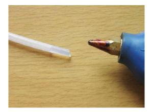
Perhaps the easiest way to make a tail is to use a short length of spiral wrap. If you don't have spiral wrap then you can make some by feeding a drinking straw through a pencil sharpener. The pencil sharpener will probably need a new blade as it has to be sharp.
