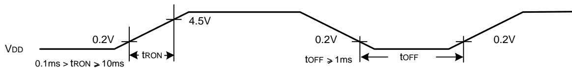
Figure 4. t_{OFF} stipulates the time of power OFF for instantaneous power supply to or when power supply repeats ON and OFF.
