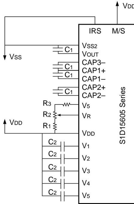
② When the voltage regulator circuit and V/F circuit alone are used
