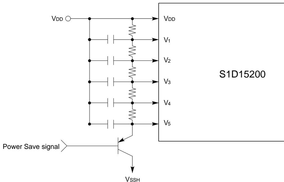
If the LCD drive power is generated by resistance division, the resistance and capacitance are determined by the LCD panel size. After the panel size has been determined, reduce the resistance to the level where the display quality is not affected and reduce the power consumption using the divider resistor.
