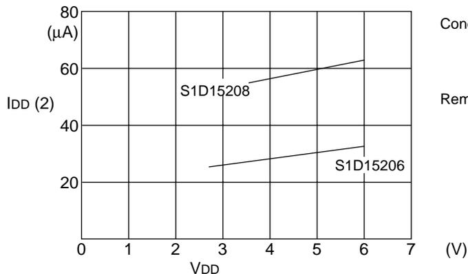
Conditions: The built-in power supply is ON.
