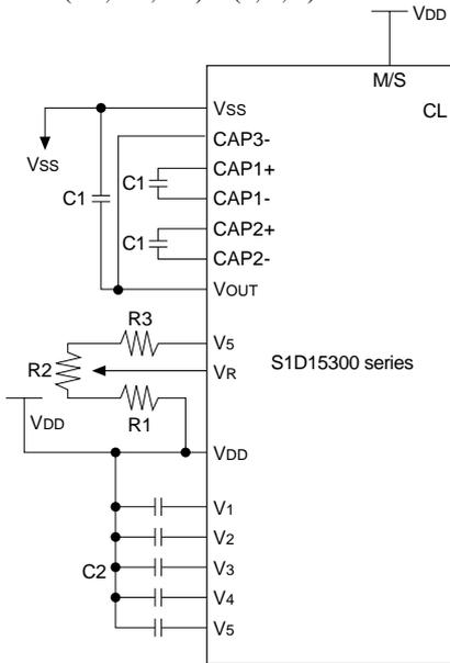
①-2 when the on-chip power circuit is used    ② when VOUT is input from the outside
