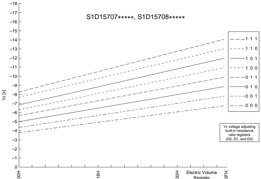
Fig. 10-2 S1D15707\*\*\*\*\*, S1D15708\*\*\*\*\* Temperature gradient = -0.05%/°C device
