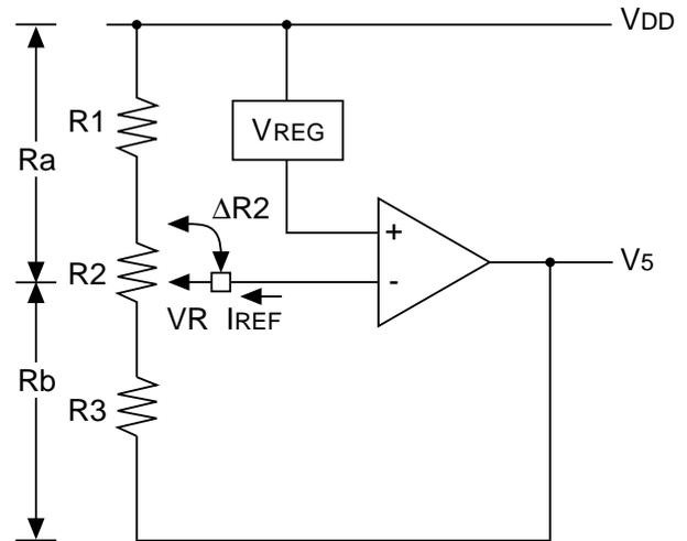
VREG is the constant voltage source of the IC, and it is constant and  $V_{REG} \doteq -2.5 \pm 0.15$  V (if VDD is 0 V). To adjust the V5 output voltage, insert a variable resistor between VR, VDD and V5 as shown. A combination of R1 and R3 constant resistors and R2 variable resistor is recommended for fine-adjustment of V5 voltage.
