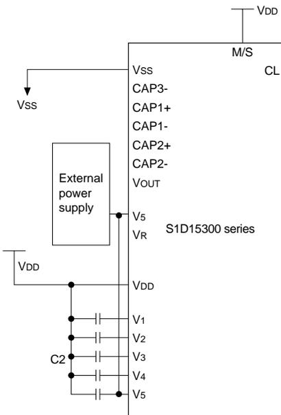
④ when the on-chip power circuit is used
