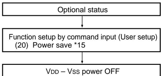
Set the time ( $t_L$ ) from power save to turning off the  $V_{DD} - V_{SS}$  power ( $V_{DD} - V_{SS} = 1.8\text{ V}$ ) longer than the time ( $t_H$ ) when the potential of  $V_5 \sim V_1$  becomes below the threshold voltage (approximately 1V) of the LCD panel.
