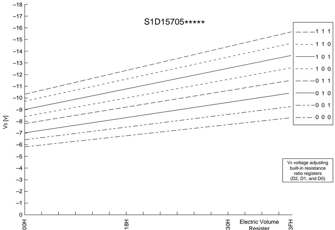
Fig. 10-1 S1D15705\*\*\*\*\* Temperature gradient = -0.05%/°C device
