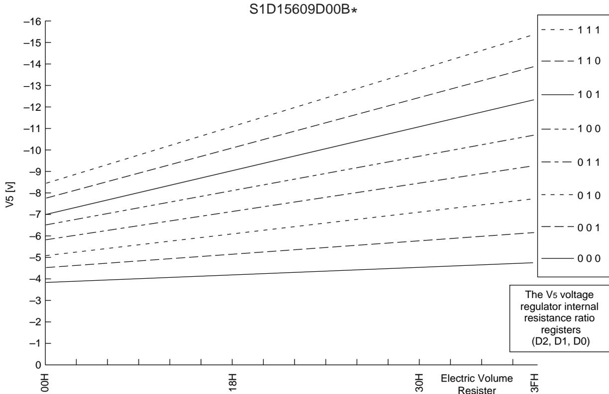
Figure 19: S1D15609D00B\* Temperature Gradient =  $-0.05\%/^{\circ}\text{C}$  Model
