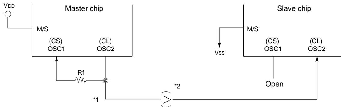
\*1 If the parasitic capacitance of this section increases, the oscillation frequency may shift to the lower frequency. Therefore, the Rf oscillation frequency must be reduced below the specified level.
