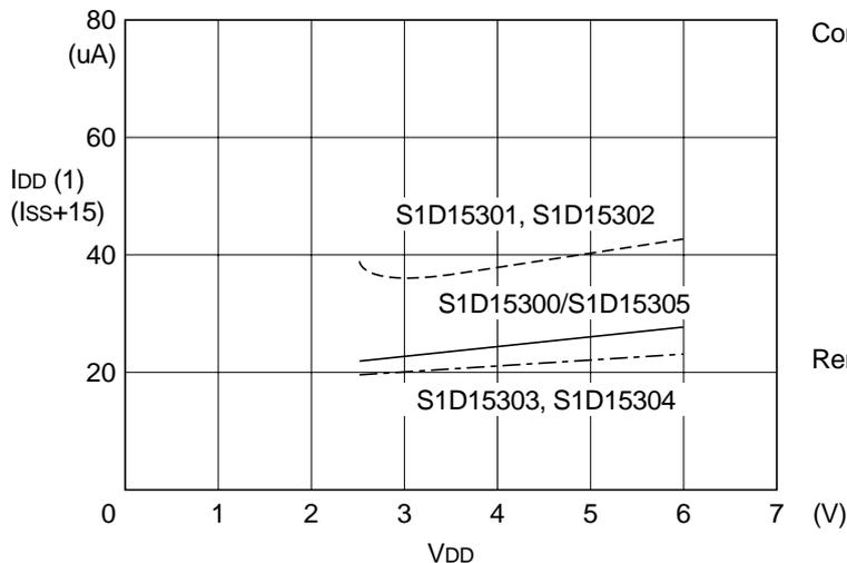
Condition: The built-in power supply is OFF and an external power supply is used.
