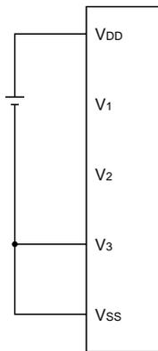
Figure 1. LCD drive supply connected to VSS
