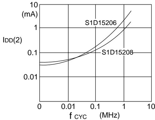
It shows the current consumption when a checker pattern is always written in fSYNC timing. When not accessed, only the current consumption of  $I_{DD}$  (2) occurs.
