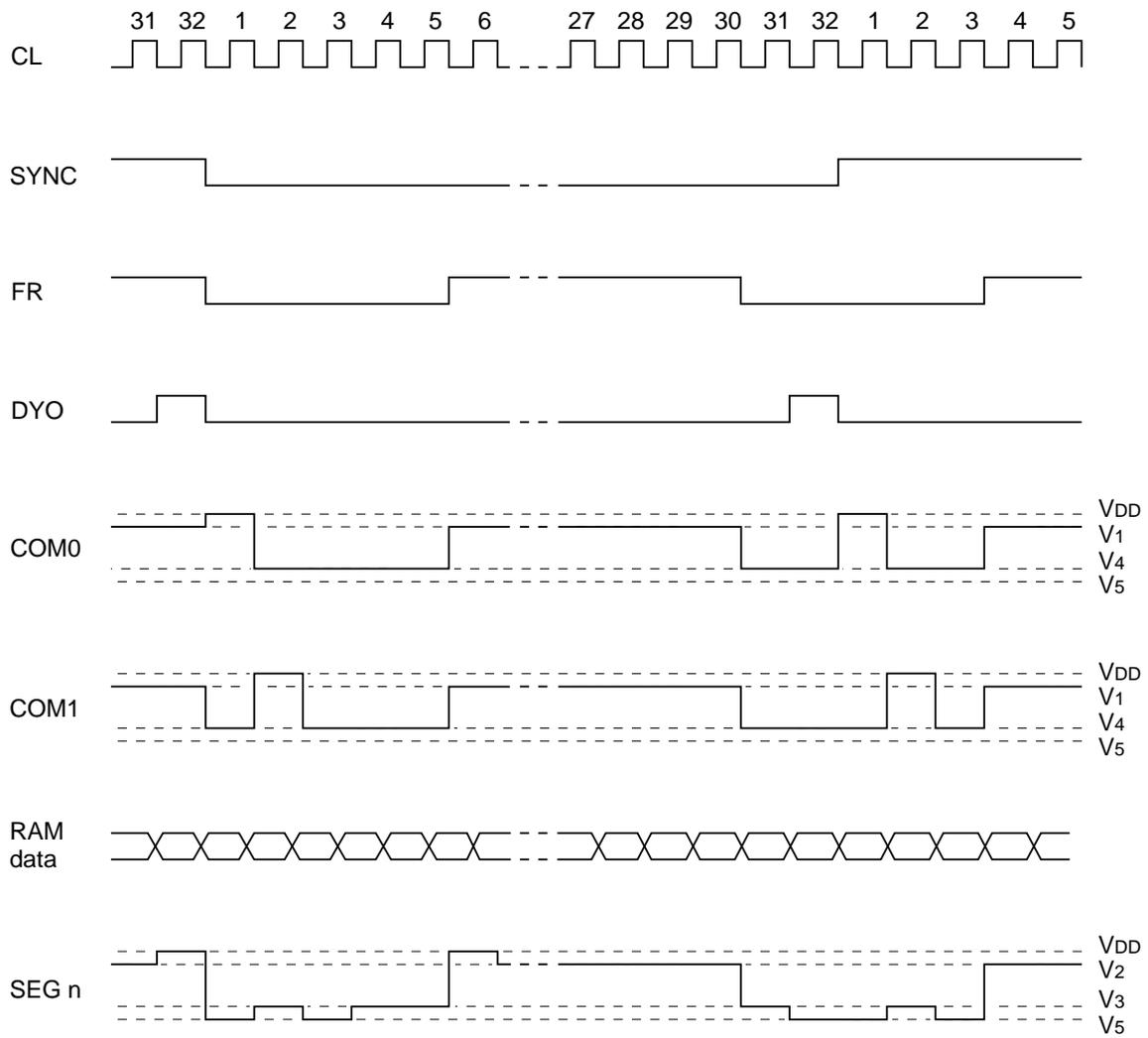
Figure 8. Line inverse driver timing
