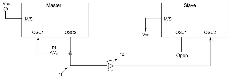
\*1 Oscillating frequency shifts to low frequency side when parasitic capacity gets larger, So Rf should be smaller than the regular value.
