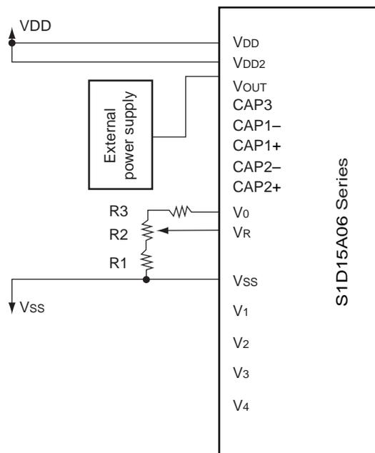
(2) When built-in  $V_0$  voltage adjusting resistors are used Voltage Follower Circuit [S1D15A06D01B\*]
