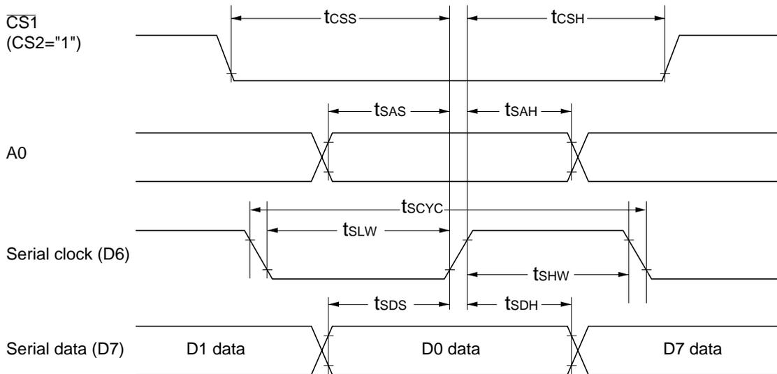
$V_{SS} = 0\text{ V}$ ,  $V_{DD} = 5.0\text{ V} \pm 10\%$ ,  $T_a = -40\text{ to }+85^\circ\text{C}$
