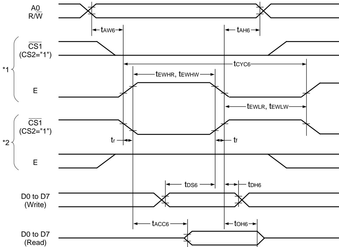
[S1D15705\*00\*\*, S1D15707\*00\*\*, S1D15708\*00\*\*: V<sub>DD</sub>=4.5V to 5.5V, T<sub>a</sub>=-40 to 85°C]
