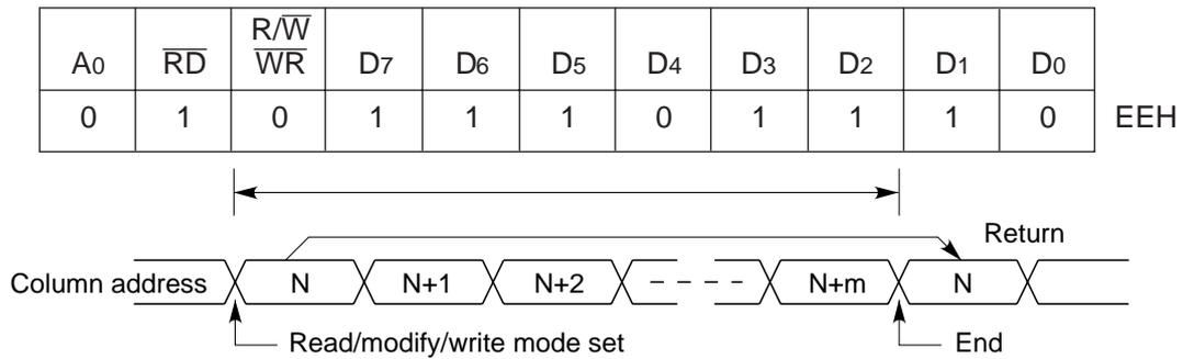
Cancels read-modify-write mode and restores the contents of the column address register to their value prior to the receipt of the read-modify-write command.
