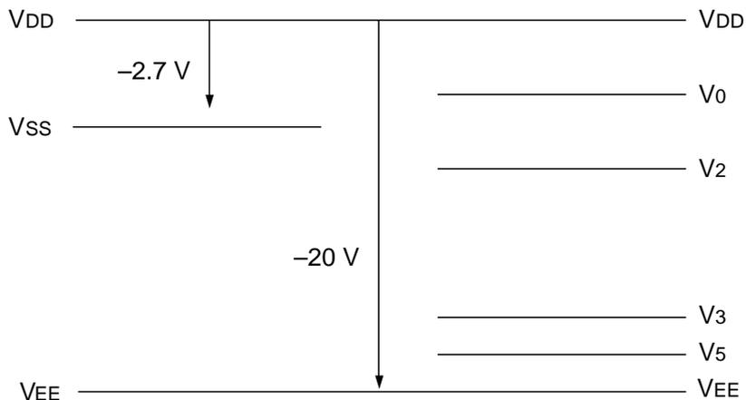
4. If the logic power is being floated or if the VSS voltage exceeds -2.5 Vdc during LCD power-on, the LSI chips may be damaged permanently. Take care not to damage the chips especially in the system power on/off sequence.
