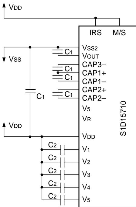
(2) When not using the V5 voltage adjusting built-in resistor (Example of Vss2=Vss, quadruple boosting)
