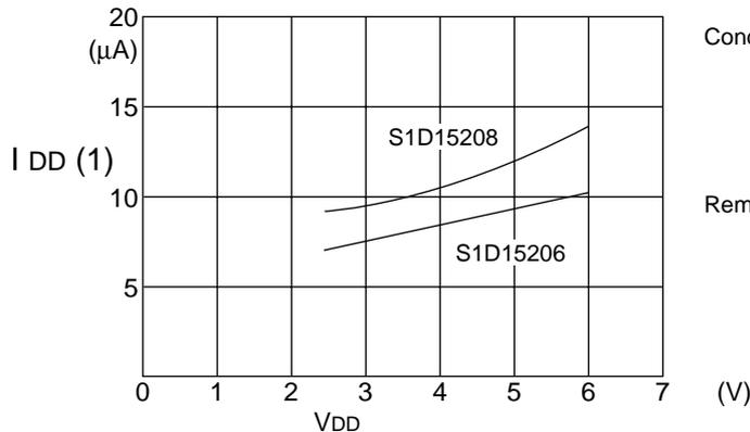
Conditions: The built-in power supply is OFF and an external power supply is used.
