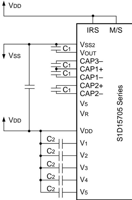
(2) When not using the V5 voltage adjusting built-in resistor
