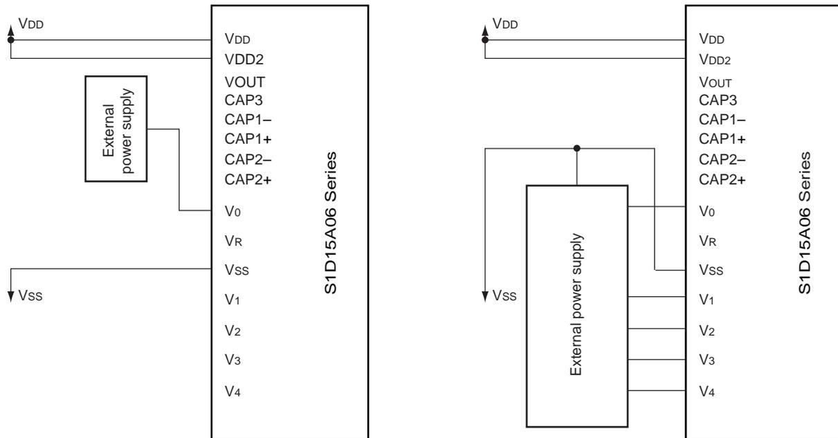
\* Since V<sub>R</sub> pin has a higher impedance, wiring distance must be minimized or shielded wire must be used.
