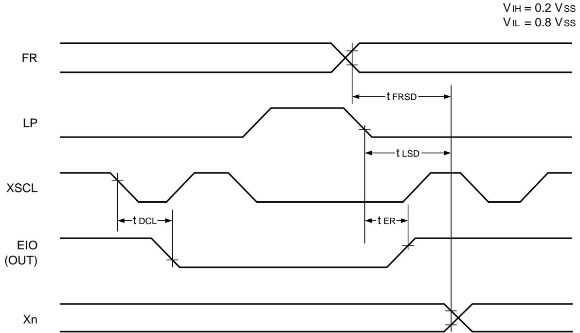
$V_{DD} = -5.0 \pm 10\%$ ,  $V_{EE} = -8.0$  to  $-20.0$  V,  $T_a = -40$  to  $85^\circ\text{C}$
