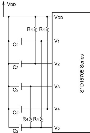
Adjust resistance value R4 to the optimal level by checking driving waveform displayed on the LCD.
