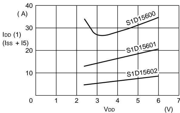
Conditions: The built-in power supply is off but the external one is used.
