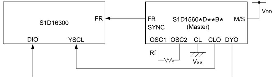
S1D1560\*D\*\*B\*-S1D1560\*D\*\*B\* (when oscillator circuit is used)
