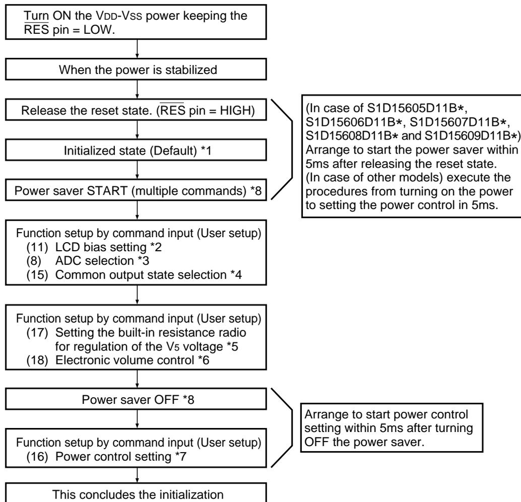
\* The target time of 5ms will result to vary depending on the panel characteristics and the capacitance of the smoothing capacitor. Therefore, we suggest you to conduct an operation check using the actual equipment.
