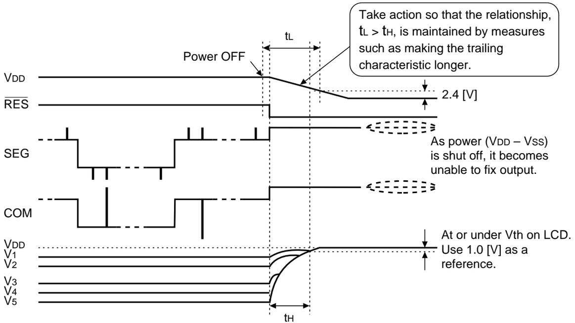
If command control is disabled when power is OFF, take action so that the relationship,  $t_L > t_H$ , is maintained by measures such as making the trailing characteristic of power ( $V_{DD} - V_{SS}$ ) longer.
