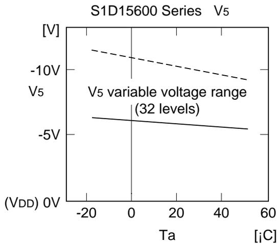
According to the  $V_5$  voltage and temperature change, equation ③ can be as follows (if  $V_{DD} = 0$  V reference):
