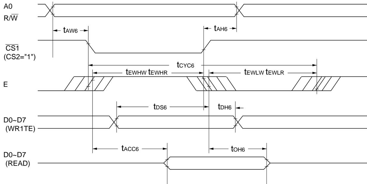
$V_{DD} = 5.0 V \pm 10\%$ ,  $T_a = -40$  to  $+85^\circ C$
