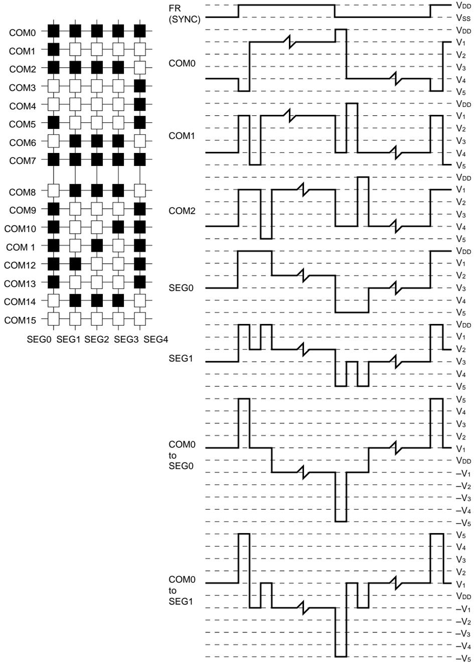
Figure 9. Example of segment and common timing
