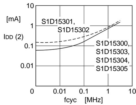
This indicates current consumption when data is always written on the checker pattern at  $fcyc$ . When no access is made, only  $I_{DD} (1)$  occurs.
