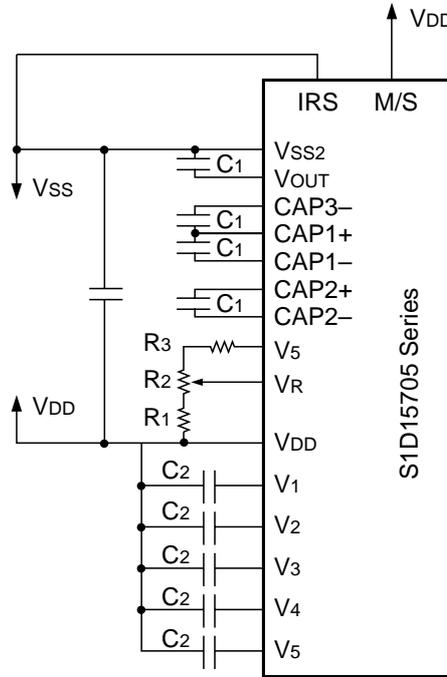
② Only the voltage adjusting circuit and V/F circuit used
