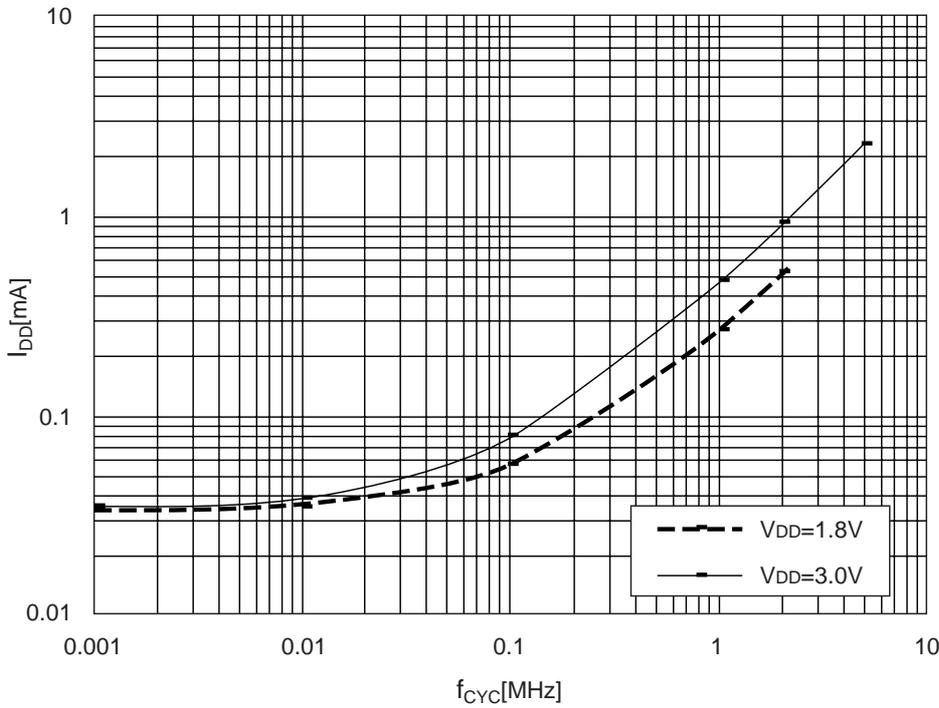
This chart shows current consumption when the checker pattern write is constantly implemented in  $f_{CYC}$ .  $I_{SS}$  (1) alone is consumed when an access is not taking place.
