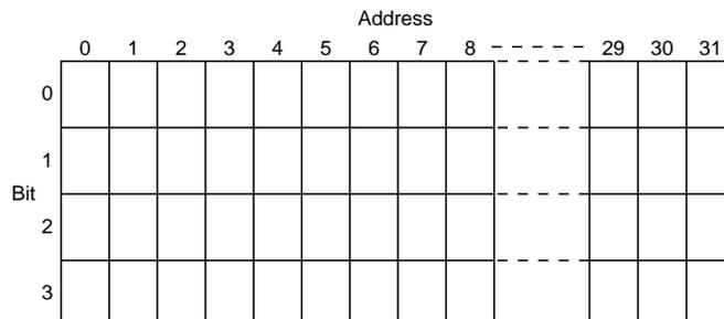
Each 8-bit display data byte loaded from the command/data register is stored in two consecutive addresses as shown in the following figure. The upper four bits are stored at the location specified by the address counter, and the lower four bits, at the next location. The address counter is automatically incremented by two.
