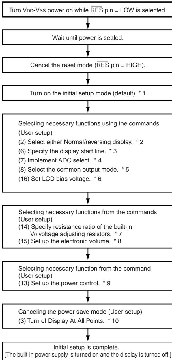
on the display screen during its powering on process. In order to avoid such troubles, it is recommended to implement the following flow.
