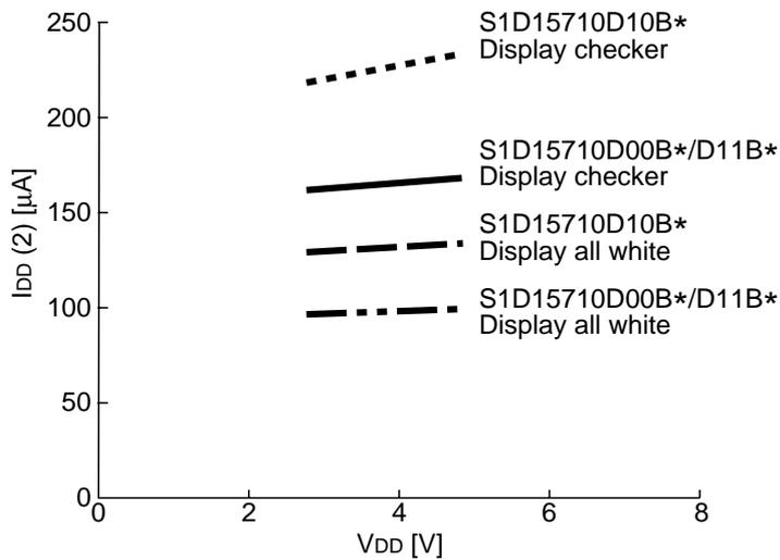
Condition: Built-in power supply ON
