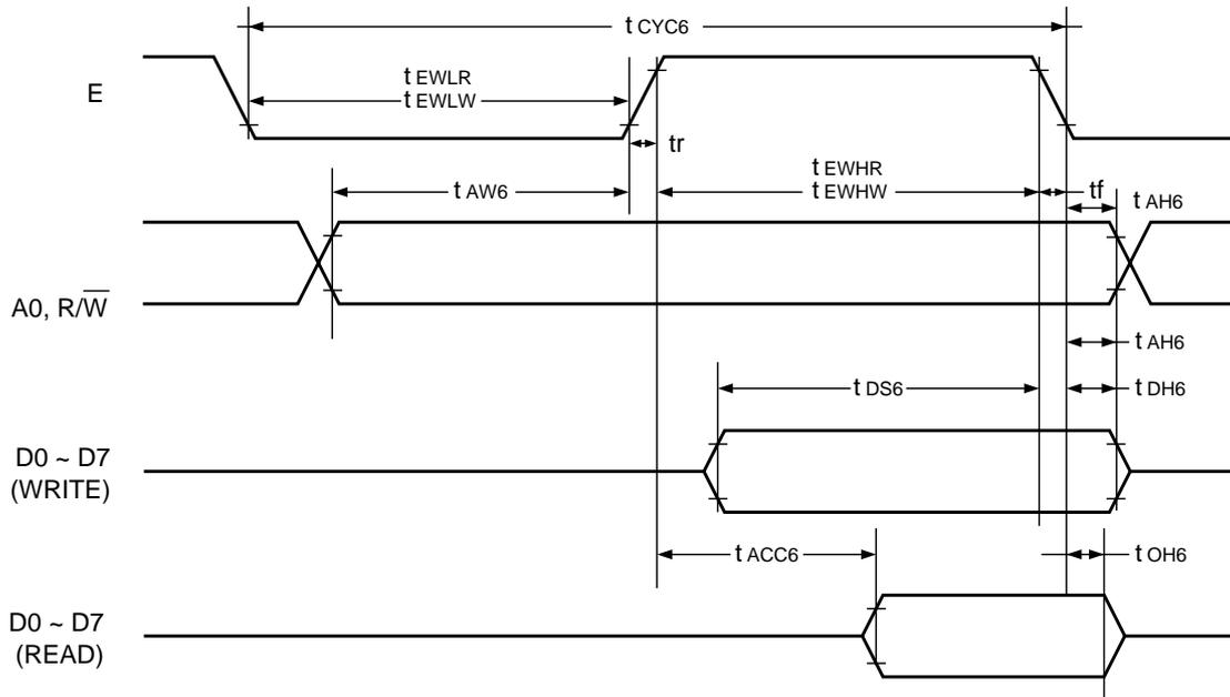
$V_{SS} = -5.0 \text{ V} \pm 10\%$ ,  $T_a = -30 \sim 85 \text{ }^\circ\text{C}$
