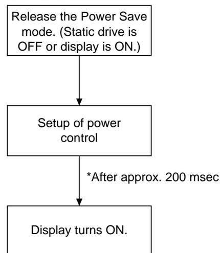
\* When the Set Power Control command is issued, the V<sub>DD</sub> level signal is output at both COM and SEG terminals for approximately 200 msec. Any other command can be entered during this period.
