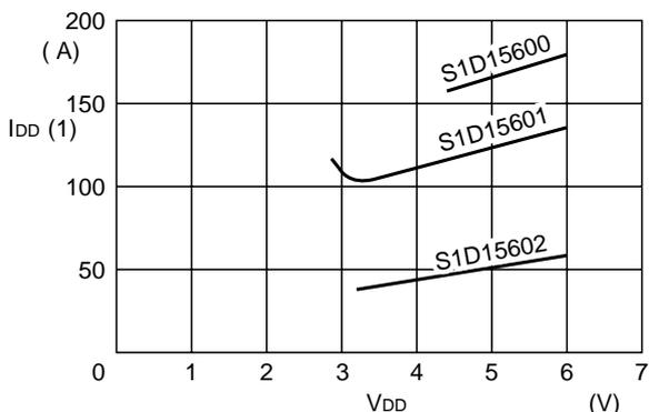
Conditions: The built-in power supply is on and T1 = T2 = Low.
