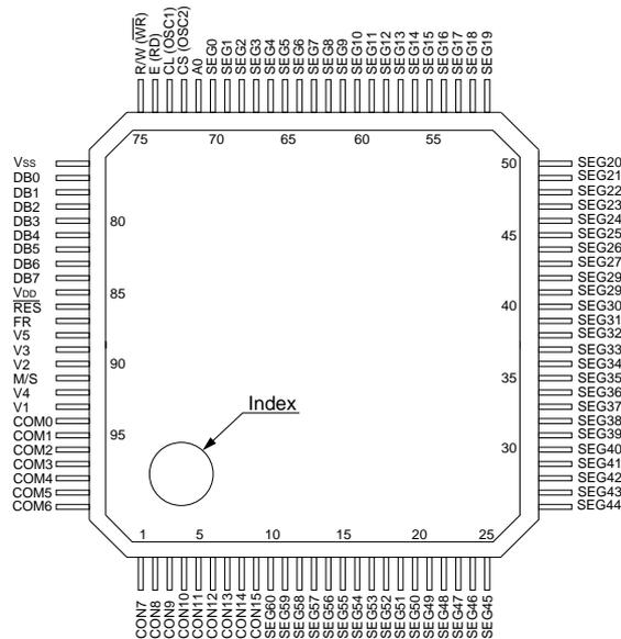
Note: This is an example of S1D15200F pin assignment. The modified pin names are given below.
