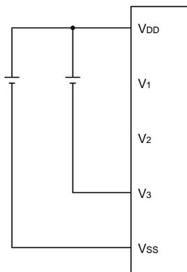
Figure 2. LCD drive supply not connected to VSS
