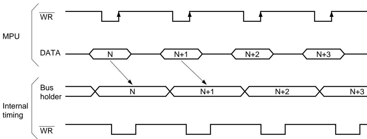
Figure 2. Write timing
