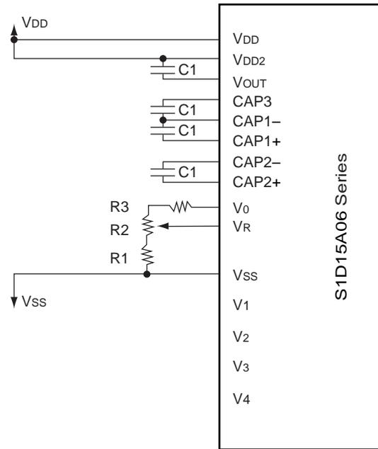
2. When the voltage adjustment and V/F circuits alone are used
