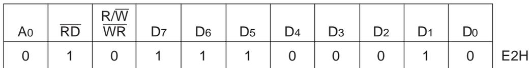
When the power supply is turned on, a Reset signal is entered in the  $\overline{RES}$  pin. The Reset command cannot be used instead of this Reset signal.
