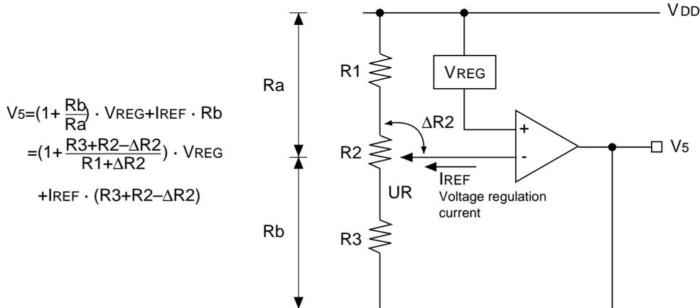
$$V_5 = \left(1 + \frac{R_b}{R_a}\right) \cdot V_{REG} + I_{REF} \cdot R_b$$
