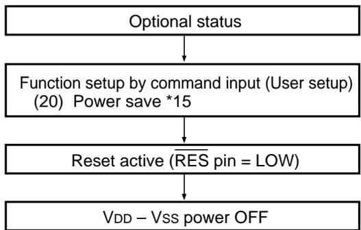
Set the time ( $t_L$ ) from reset active to turning off the  $V_{DD} - V_{SS}$  power ( $V_{DD} - V_{SS} = 1.8\text{ V}$ ) longer than the time ( $t_H$ ) when the potential of  $V_5 \sim V_1$  becomes below the threshold voltage (approximately 1 V) of the LCD panel. For  $t_H$ , refer to the <Reference Data> of this event. When  $t_H$  is too long, insert a resistor between  $V_5$  and  $V_{DD}$  to reduce it.
