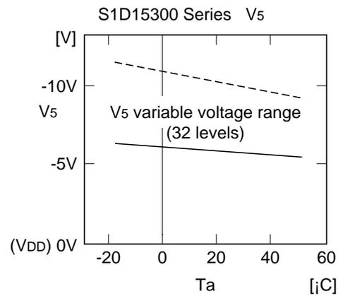
According to the  $V_5$  voltage and temperature change, equation ⑤ can be as follows (if  $V_{DD} = 0V$  reference):
