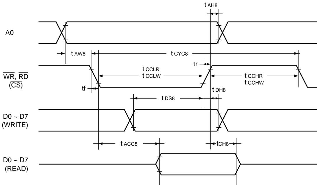
V<sub>SS</sub> = -5.0 ± 10%, T<sub>a</sub> = -30 to 85 °C
