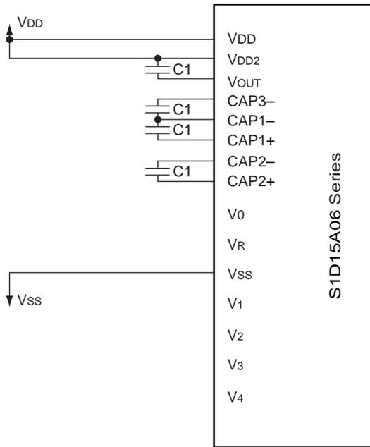
(2) When built-in  $V_0$  voltage adjusting resistors are not used (When  $V_{DD2} = V_{DD}$  boosted 4 times)
