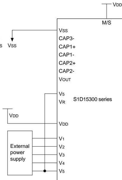
Reference setup value: S1D15300  $V_5 \approx -7$  to  $-9$  V
